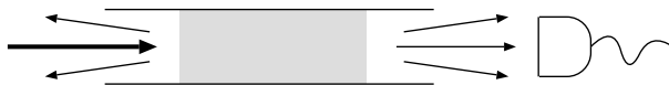
Figure 2.1: Coherent light (thick arrow) is incident on an amplifying medium (shaded), embedded in a waveguide. The transmitted radiation is measured by a photodetector.
