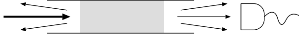
Figure 3.1: Schematic illustration of direct detection: Radiation is incident on a random medium (shaded). The transmitted radiation is absorbed by a photodetector.
