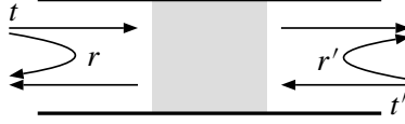
Figure 1.3: The scattering matrix S can be decomposed into transmission matrices ( t and t' ) and reflection matrices ( r and r' ).
