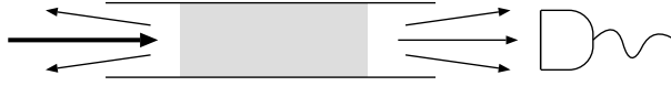
Figure 4.1: Coherent light (thick arrow) is incident on an absorbing or amplifying medium (shaded), embedded in a waveguide. The transmitted radiation is measured by a photodetector.
